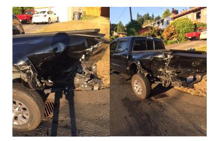
Repairs of the vehicle included extensive frame/unibody repairs and body work and painting on extensive areas of the vehicle. The total repair cost was \$17,735.79.
